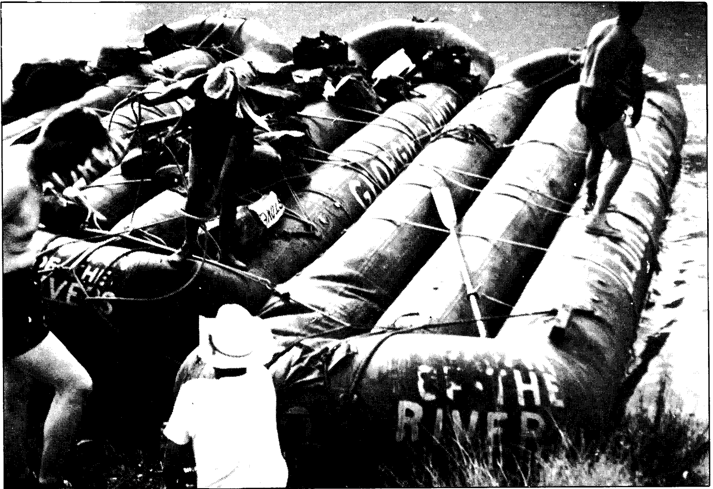
Georgie's triple pontoon rig ("big boat") on her 1957 river trip from Green River, Utah, to Hite. Georgie is in the process of reversing the side pontoon. Note the deflated front chamber suffered from a stick that tore the fabric while going to shore. Photography by L. C. B. McCullough. Photo courtesy of Rosalyn Jirge.
